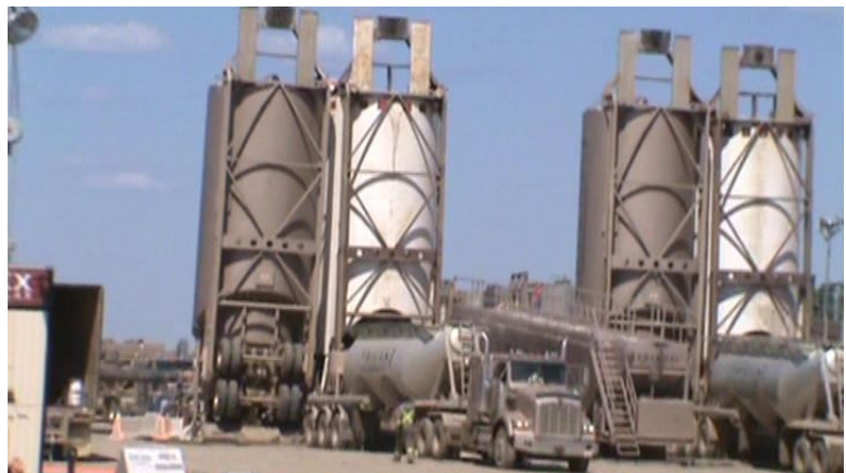
Here, frack sand containers at the 2 Island Operation are hauled to the fracking site and erected into standing towers to allow the frack sand to empty freely by gravity.
