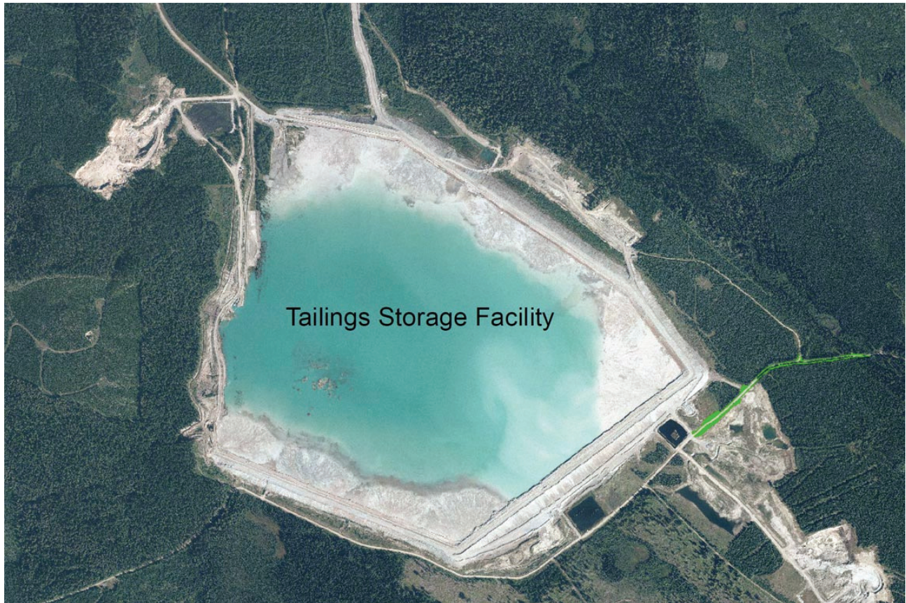
Above: an undated aerial photo used in Figure 7.1, Disturbed and Reclaimed Surfaces 2011 , in the 2011 Annual Environmental and Reclamation Report . Note the location of the supernatant pond adjoining half the mid-crest length of the Main Embankment. The configuration of the pond is roughly similar to the May 15, 2010 satellite image above.
