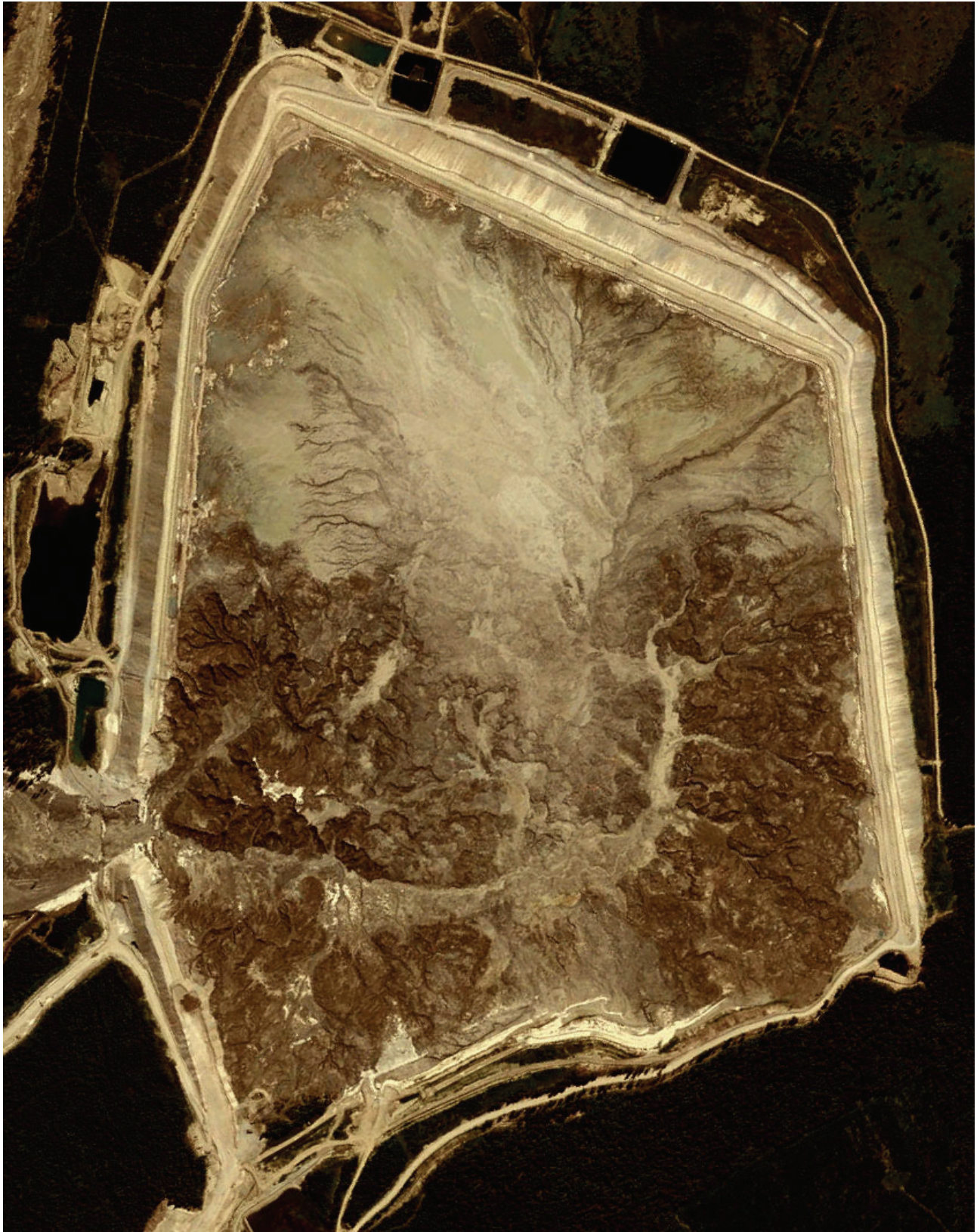
Photoshop rendering of Google Earth satellite image of Mount Polley TSF, using “neutrals” variable settings in “selective color” adjustment in Photoshop, to better highlight the saturated mass tailings implosion flow exit paths, dendritic drainage patterns, and lateral stress forces. The darker brown areas denote the depleted and collapsed tailings mass, while the lighter zone on the top half shows the compressed tailings mass.
